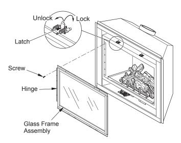
Figure 42 - Removing/Replacing Glass Door
